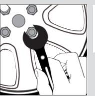
Lug nuts are evenly tightened to manufacturer's specification to ensure an optimum ride, prevent rotor warpage and ease removal.
